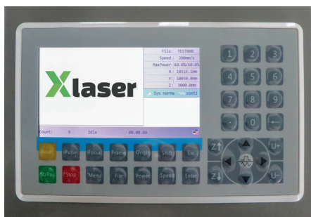
DSP Control System
